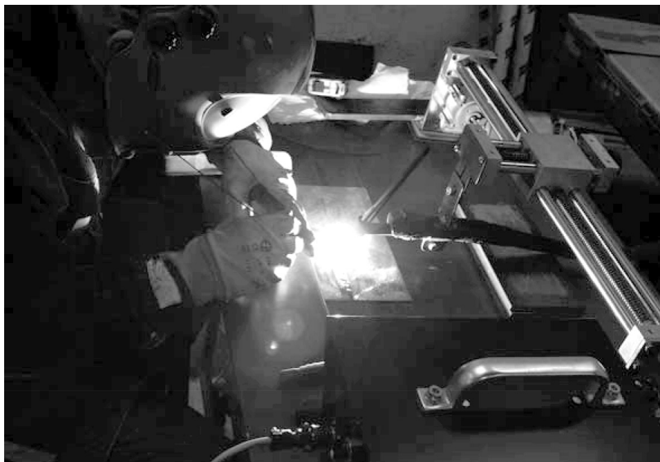
Fig. 1. Weld overlay with automated movement of the welding torch
