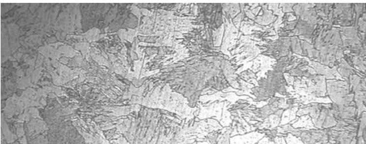
**Fig. 11.** Microstructure of remelted strip, ITIG,  $\times 100$
