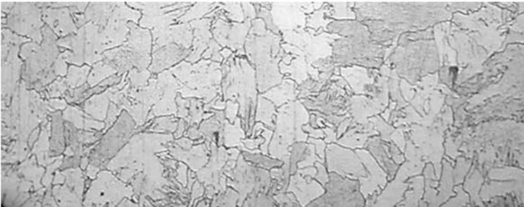
**Fig. 10.** Microstructure of remelted strip, TIG,  $\times 100$
