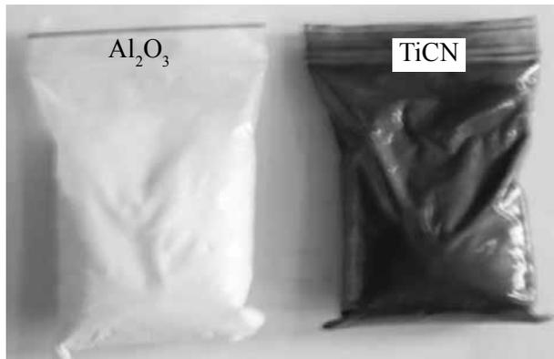
**Fig. 1.** Nanopowders of  $\text{Al}_2\text{O}_3$  and  $\text{TiCN}$  with size 45–55 nm
