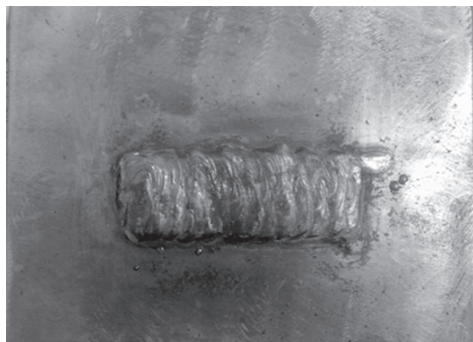
Fig. 1. Surfaced layer on steel with 25 mm thickness
