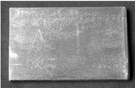
Fig. 1. Abrasively cleaned and degreased sample surface
