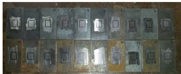
Figure 3. Plates prepared for weld overlay of coatings
