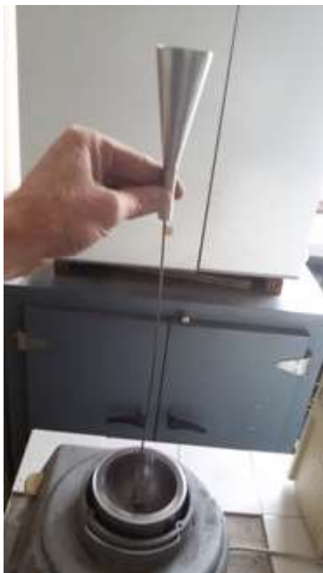
Figure 1. Vibration filling of cored wires
