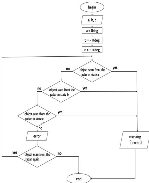
Fig. 12. Algorithm block diagram of the code for radar scanning process.
