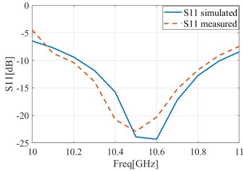
Fig. 4. S parameters of simulated and fabricated patches
