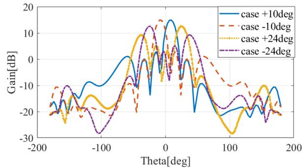
Fig. 11. Radiation Pattern in scanning modes on H plane (Azimuth)
