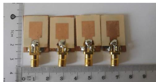
Figure 2. Fabricated patches for antenna array
