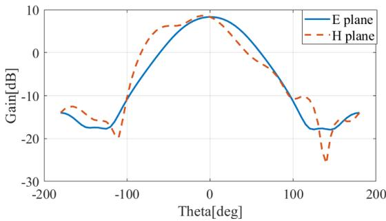
Fig. 5. Radiation pattern of patch antenna (measured)
