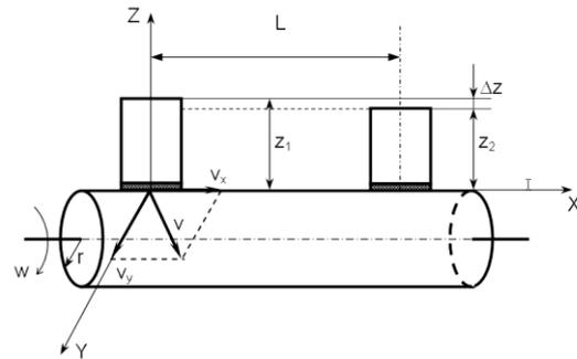
Figure 2: Sketch of the velocity of contact area center
