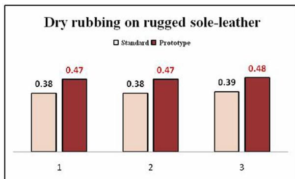
Fig. 5. Static friction coefficient on rugged sole-leather under load: 1 - 19,4 N; 2 - 38,8 N; 3 - 58,2 N.
