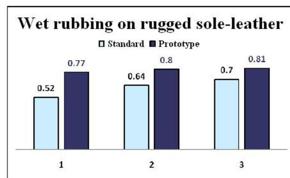
Fig. 9. Static friction coefficient on a rugged sole-leather under load: 1 - 19,4 N; 2 - 38,8 N; 3 - 58,2 N,
