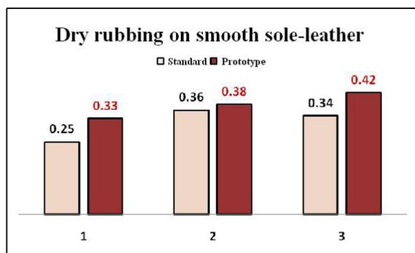
Fig. 6. Static friction coefficient on smooth sole-leather under load: 1 - 19,4 N; 2 - 38,8 N; 3 - 58,2 N
