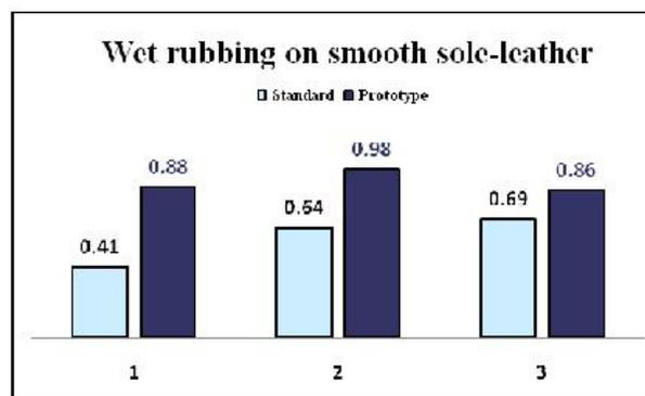
Fig. 10. Static friction coefficient on a smooth sole-leather under load: 1 - 19,4 N; 2 - 38,8 N; 3 - 58,2 N.
