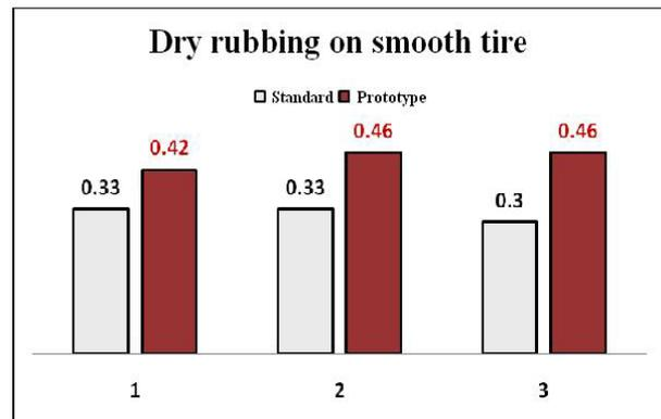
Fig. 4. Static friction coefficient on a smooth tire under load: 1 - 19,4 N; 2 – 38,8 N; 3 – 58,2 N.
