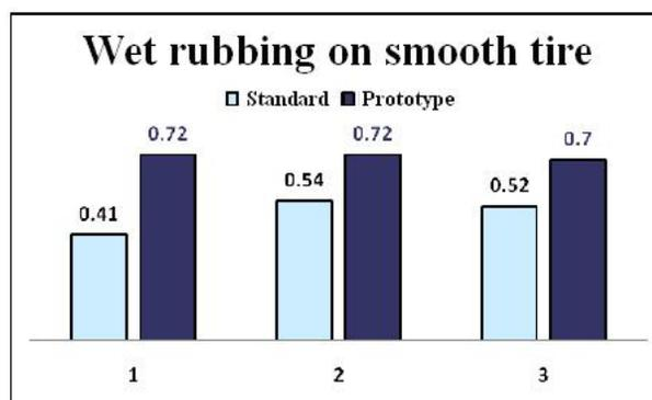
Fig. 8. Static friction coefficient on a smooth tire under load: 1 - 19,4 N; 2 - 38,8 N; 3 - 58,2 N
