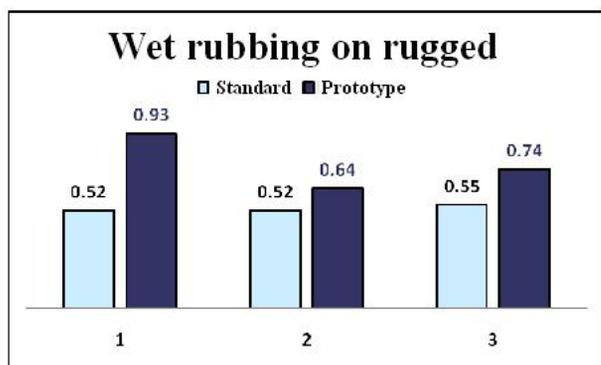
Fig. 7. Static friction coefficient on a rugged tire under load: 1 - 19,4 N; 2 - 38,8 N; 3 - 58,2.
