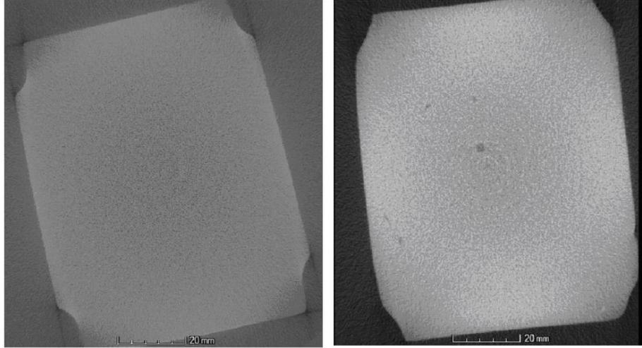
Fig. 2. Nondestructive benchmarking of the internal structure top view - a) prototype (“new” model); (b) benchmark (“old” model).
