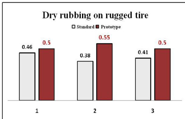
Fig. 3. Static friction coefficient on a rugged tire under load: 1 - 19,4 N; 2 – 38,8 N; 3 – 58,2 N.
