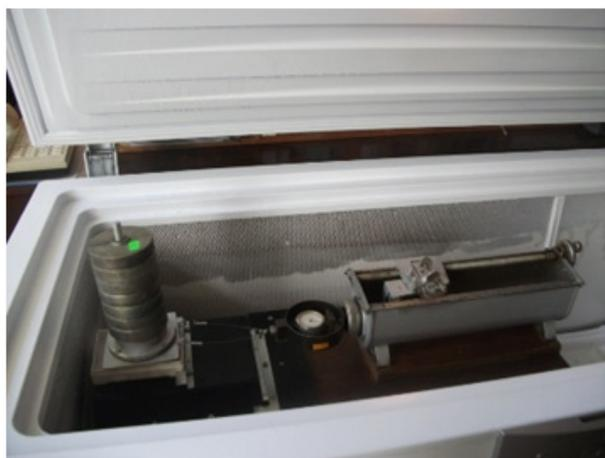
Fig. 2. Photograph of the tribological tester placed into a cryogenic camera.
