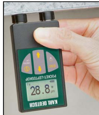
Figure 3. Pocket Leptoskop 2021Fe.
