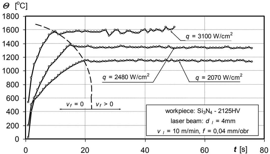
Fig. 6 Surface temperature of Si<sub>3</sub>N<sub>4</sub> ceramics while laser heating of the workpiece along the helical line with various power density  $q$
