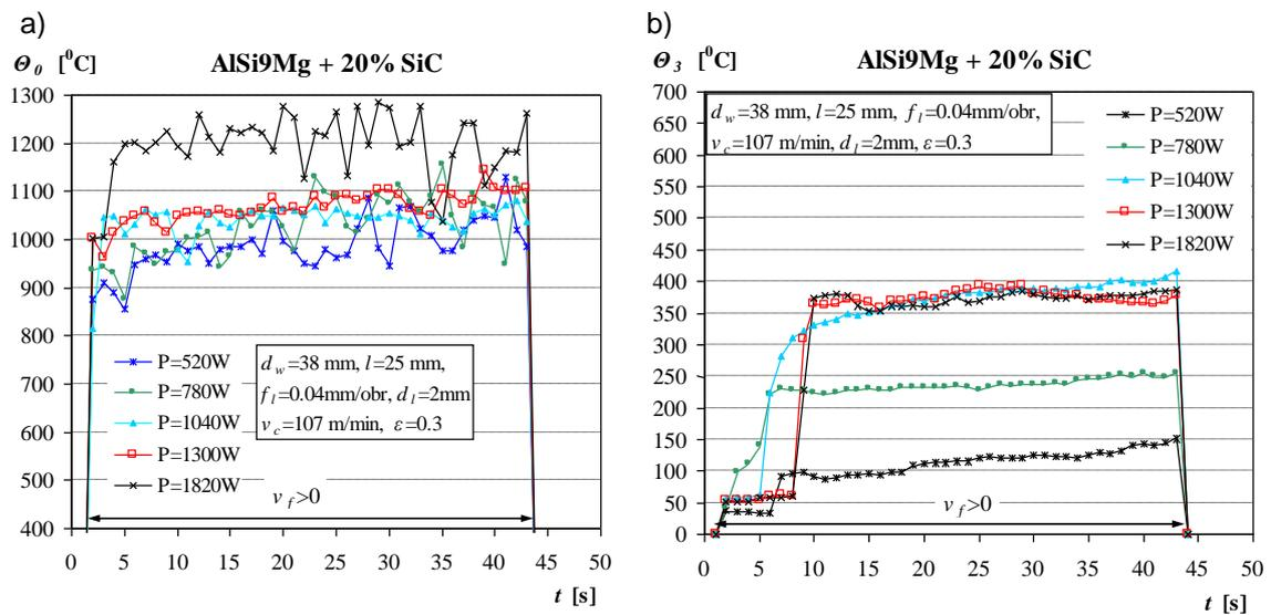
Fig. 8 Comparison of measured temperatures with different power of laser beam, a) measured from  $\theta_0$  area, b) measured from  $\theta_3$  area
