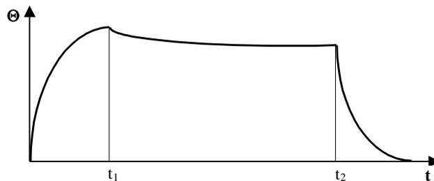
Fig. 1 Particular phases of the laser heating of the Si<sub>3</sub>N<sub>4</sub> ceramics
