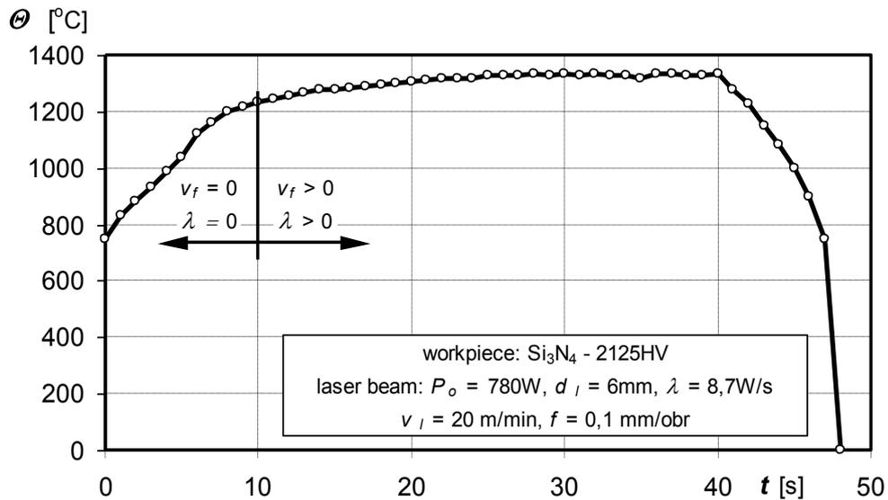
Fig. 7 Surface temperature of Si<sub>3</sub>N<sub>4</sub> ceramics while laser heating of the workpiece
