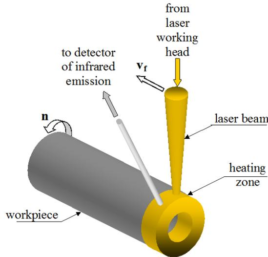
Fig. 2 Schematic process of material laser heating and remote control of measuring the surface temperature
