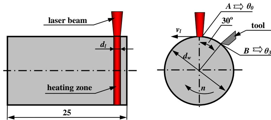
Fig. 3 Schematic of experimental set-up for metal matrix composite material. Designations: *A* - heating area by laser beam, *B* - zone of machining,  $\theta_0$ ,  $\theta_3$  - areas of temperature measurement,  $d_w$ - workpiece diameter,  $d_l$  - laser beam diameter
