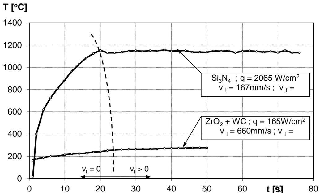
Fig. 5 Surface temperature of  $\text{Si}_3\text{N}_4, \text{ZrO}_2 + \text{WC}$  ceramics while laser heating of the workpiece along the helical line with various power density  $q$
