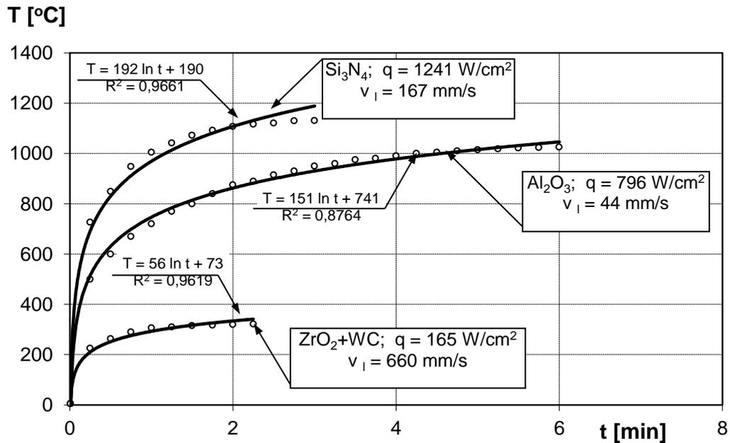
Fig. 4 Temperature  $T$  of surface sleeves made of  $\text{Si}_3\text{N}_4, \text{Al}_2\text{O}_3, \text{ZrO}_2 + \text{WC}$  vs. time  $t$  of heating by means of laser beam with various power density  $q$
