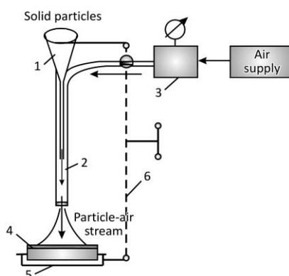
**Figure 5.** Schematic diagram of erosive wear testing.
