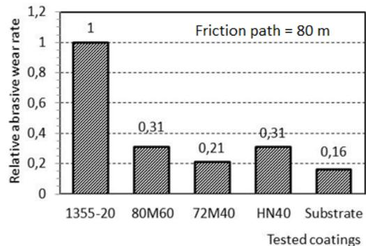
**Figure 4.** Diagram of relative wear rate to wear rate of coating with minimal wear rate (1355-20).
