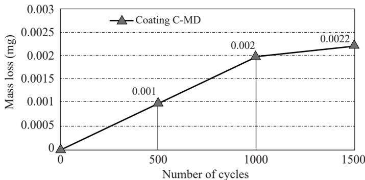
**Fig. 7.** Change in mass wear from the number of cycles/friction path for coating C-MD
