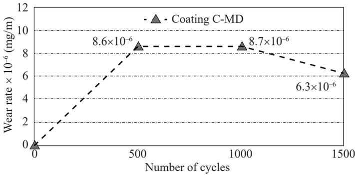
**Fig. 8.** Change in the wear rate of the number of cycles/friction path for coating C-MD
