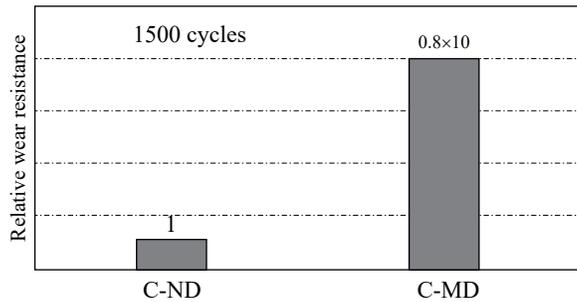
Figure 13 shows a comparative diagram of the wear resistance of coatings for the same friction path – 1500 cycles (346 m), and in Fig. 14 – the effect of the size of diamond coatings on the relative wear resistance indicator.
