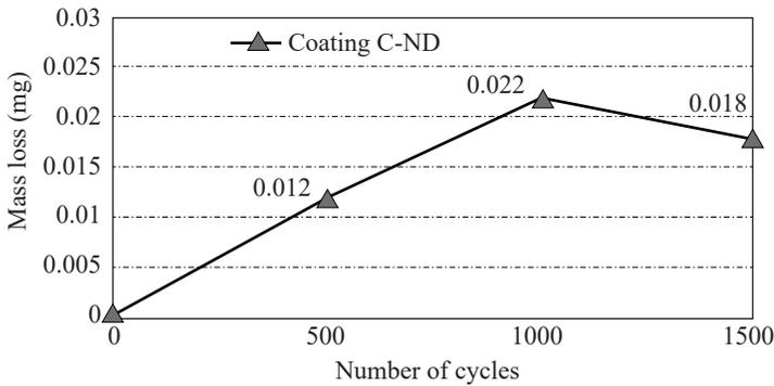
**Fig. 9.** Change in mass versus from the number of cycles/friction path for coating C-ND
