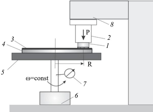
**Fig. 6.** Schematic diagram of abrasive wear testing on pin-disc tribometer
