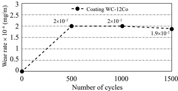
**Fig. 12.** Change in the wear rate of the number of cycles/friction path for coating WC-12Co
