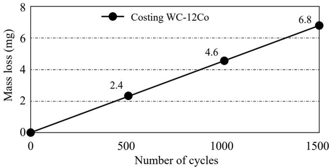
**Fig. 11.** Change in mass versus from the number of cycles/friction path for coating WC-12Co
