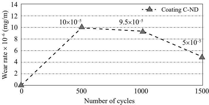
**Fig. 10.** Change in the wear rate of the number of cycles/friction path for coating C-ND
