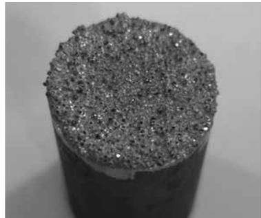
**Fig. 1.** Specimen with diamond coating
