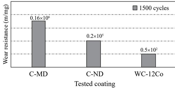
**Fig. 14.** Influence of diamond particle size on the wear resistance of coatings
