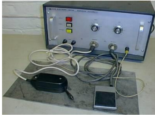
Fig. 1. Device for Manual electrical discharge deposition with vibrating electrode "Carbide Hardedge" created by Aids Electronics Ltd - England, USA
