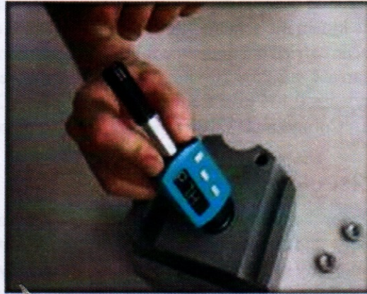
Fig. 2. Measuring of the hardness of the coatings with Bambino
