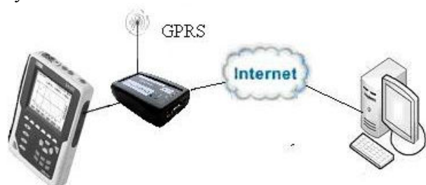
Fig. 5 Configuration for communication via GPRS
