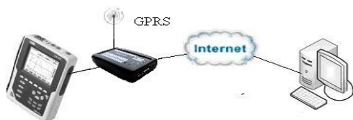
Figure 2. Configuration for communication via GPRS
