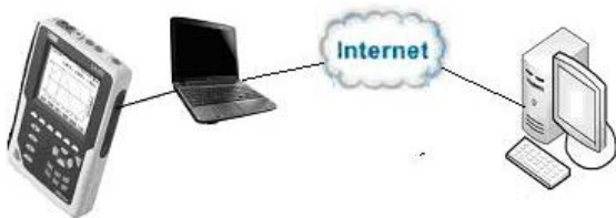
Figure 1. Configuration for communication via Ethernet
