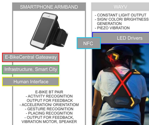
Fig.2. E-Bike- wearable LED indicator system WAVY [6] with new E-Bike – control diagram
