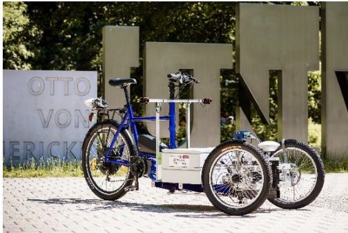
Fig.6. Autonomous urban cargo E-Bike prototype – project by Otto-von-Guericke-university Magdeburg; Photo: Jana Dünnhaupt/ OVGU
