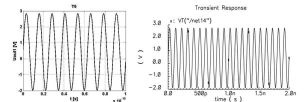
FIG. 8. FIRST OUTPUT VOLTAGE ( $U_{OUT1}$ ) VS. TIME (T).
