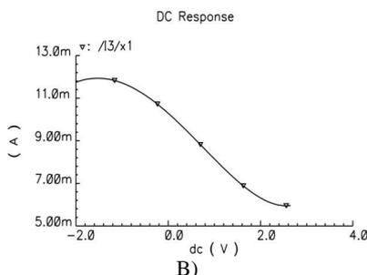
FIG. 5 OUTPUT CURRENTS (A)  $I_{OUT1}$  AND (B)  $I_{OUT2}$  VS. INPUT VOLTAGE.
