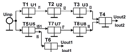
FIG. 2. MICROELECTRONIC CIRCUIT ANALOGOUS TO HYDROGEN BONDING NETWORK.
