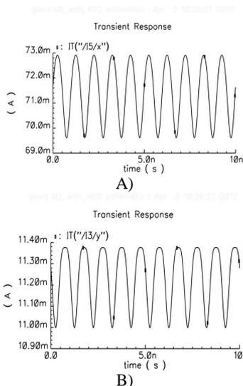
FIG. 12. OUTPUT CURRENTS (A)  $I_{OUT1}$  AND (B)  $I_{OUT2}$  VS. TIME (T) IN CADENCE.
