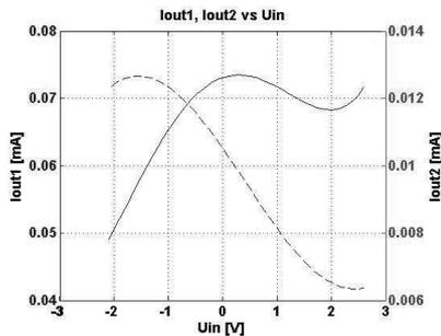
FIG. 4 OUTPUT CURRENTS ( $I_{OUT1}$  AND  $I_{OUT2}$ ) VS. INPUT VOLTAGE ( $U_{IN}$ ). WITH DASHED LINE –  $I_{OUT2}$ .
