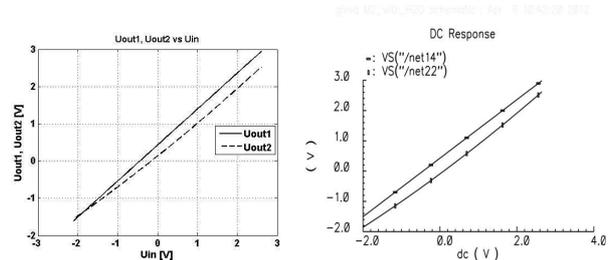
FIG. 6 OUTPUT VOLTAGES ( $U_{OUT1}$  AND  $U_{OUT2}$ ) VS. INPUT VOLTAGE ( $U_{IN}$ ) A) MATLAB AND B) CADENCE.
