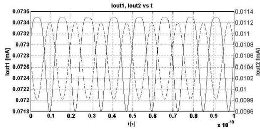
FIG. 11 OUTPUT CURRENTS ( $I_{OUT1}$  AND  $I_{OUT2}$ ) VS. TIME (T). WITH DASHED LINE –  $I_{OUT2}$  IN MATLAB.
