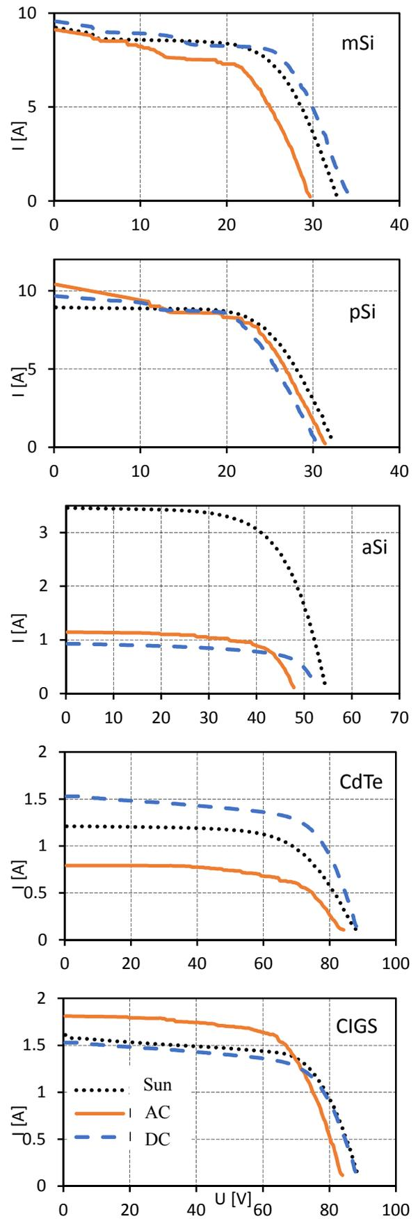
Fig. 7. IV curves of the tested PV panels under similar testing conditions with AC (orange line) and DC (blue dashed line) power supply of the solar simulator and under natural light (black dotted line).
