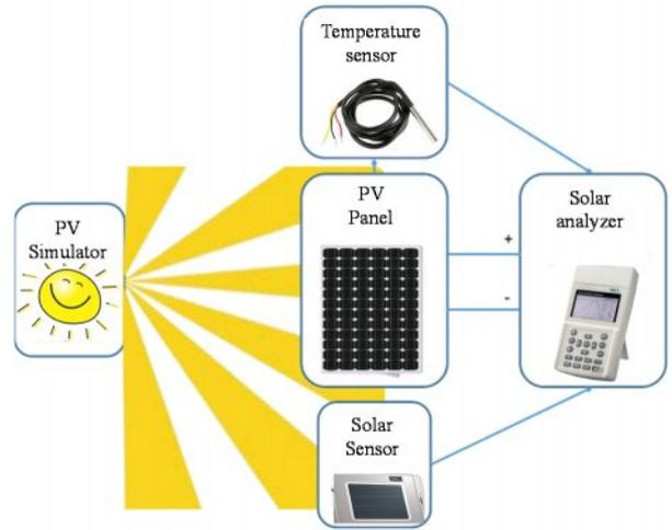
Fig. 3. Block scheme of the realized test bench
