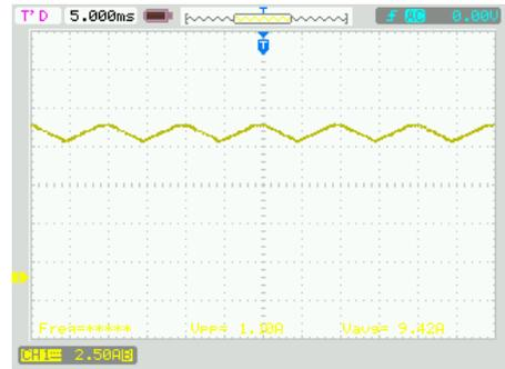
Fig. 4. Short-circuit current of the tested mSi PV panel with AC power supply of the solar simulator.
