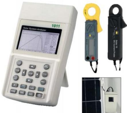
Fig. 2. Photo of the PV analyzer and its peripherals
