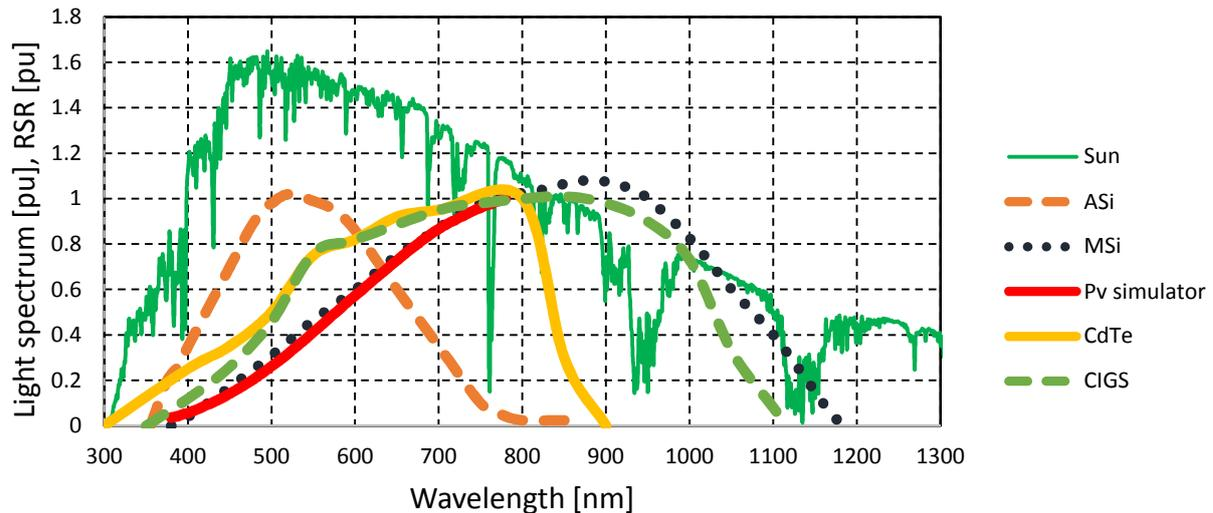
Fig. 8. Comparison of the light spectrums emitted by the Sun [5] and the solar simulator [6] and the spectral sensitivity of the tested PV panel technologies [7], [8].
