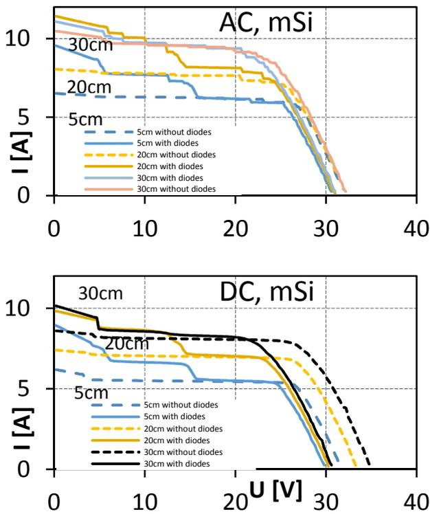
Fig. 6. IV curves of the tested mSi panel with and without protection diodes at different distances from the lightsource and different types of solar simulator's power supply.
