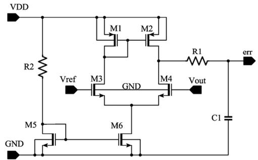
Fig. 3. Schematic of the Error amplifier.
