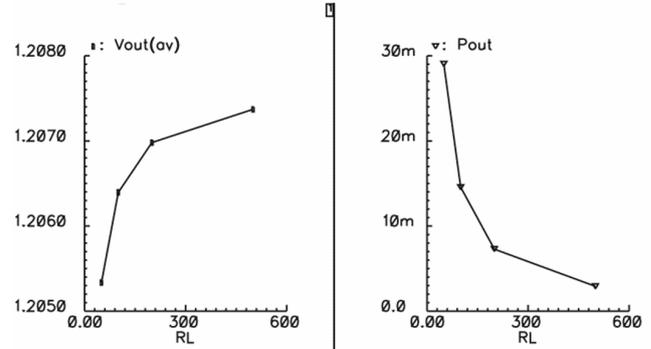
Fig. 9. Simulated load characteristic of the buck converter.
