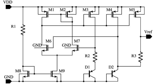
Fig. 2. Bandgap voltage reference.
