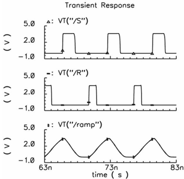
Fig. 5. Voltages of the RS flip-flop inputs and the output of ramp generator.
