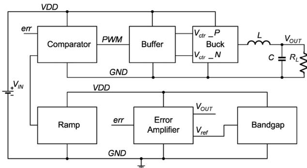
Fig. 8. Block diagram of the buck converter system.
