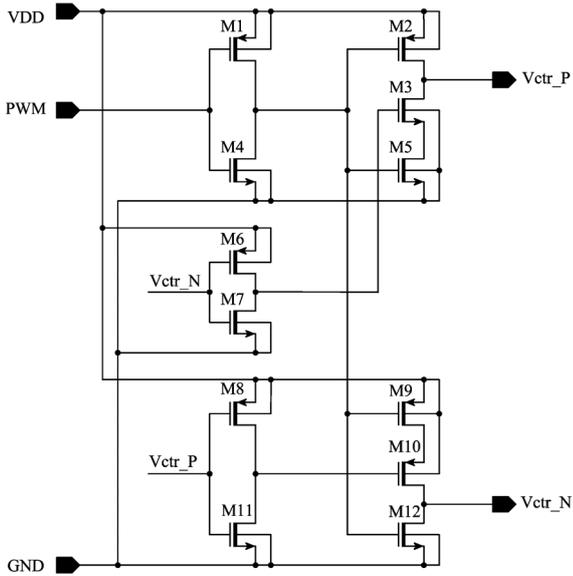
Fig. 7. Electrical schematic of the buffer, which prevents short-circuit losses.
