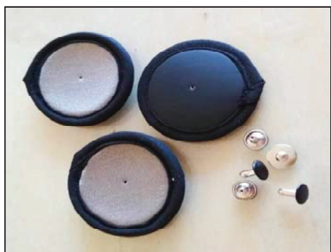
Fig. 5. Textile electrodes with edging.
