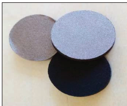
Fig. 2. Textile electrodes without edging.
