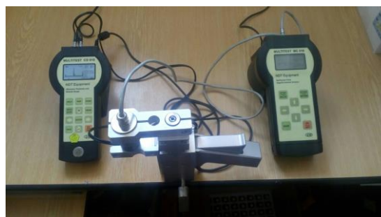
Fig. 1. System of DK100 testing jaws and MULTITEST MC010 and MULTITEST CD010 devices
