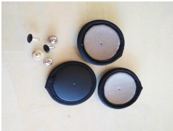
Fig. 2. Textile Electrode – Model 2 – with edge
