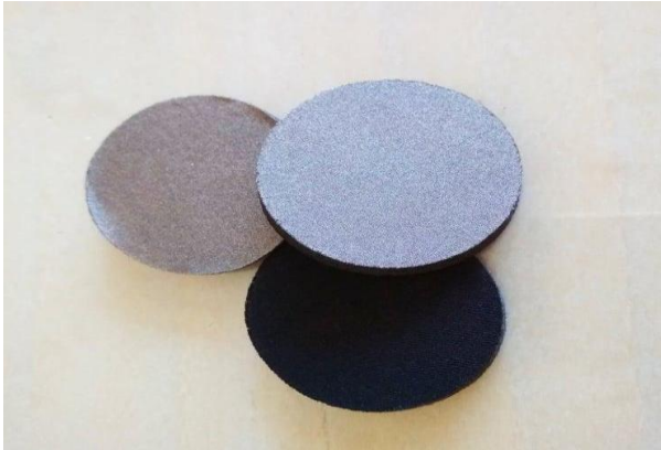
Fig. 1. Textile Electrode – Model 1 – without edge
