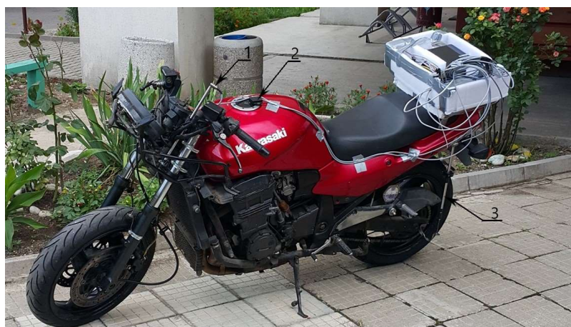
Figure 2. Kawasaki GPZ 1100 equipped with sensors and computer.
