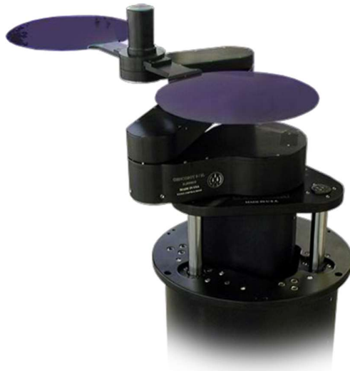
Fig. 6. Hybrid parallel-serial structure of substrate handling robots.
