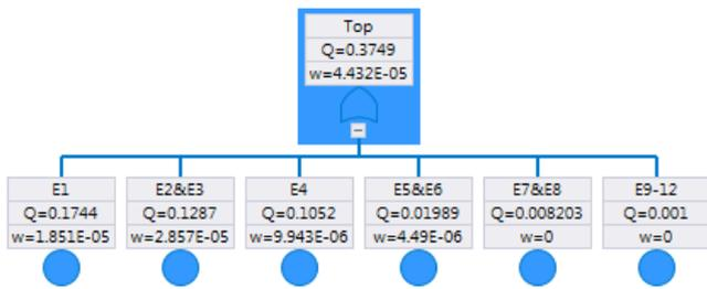
Fig. 7. Results for the unavailability of the of the variable speed induction motor drive
