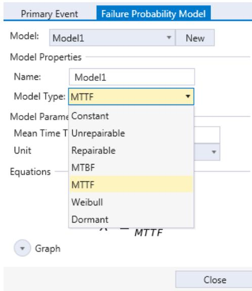
Fig. 5. Failure probability modelling functions
