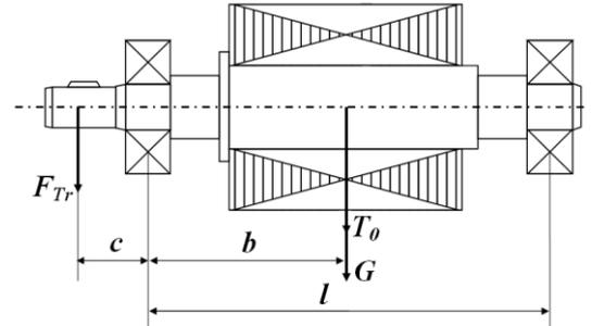
Fig. 6. Bearing dynamic load scheme
