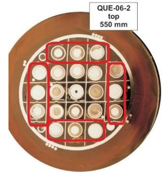
Figure 10. Bundle and fuel rods cross-section at 550 mm elevation [3].
