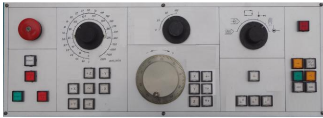
Fig. 2. Control panel for the modernized machine.
