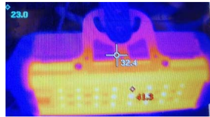
Fig. 10 Thermal image for C30 plane during light distribution measurement on MDGP
