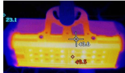
Fig. 11 Thermal image for C60 plane during light distribution measurement on MDGP
