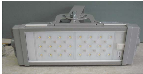
Fig. 1. Target object of the thermal imaging camera – LED luminaire
