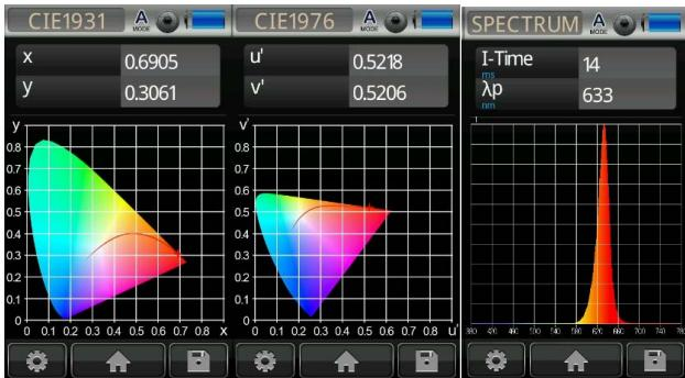
Fig. 6 Spectrum and color coordinates of the flood lights used for the “red” of the Bulgarian flag
