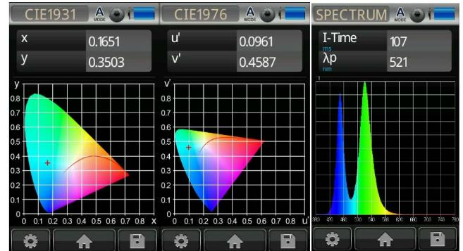
Fig. 2 Spectrum and color coordinates of the green projectors used for the colonnade
