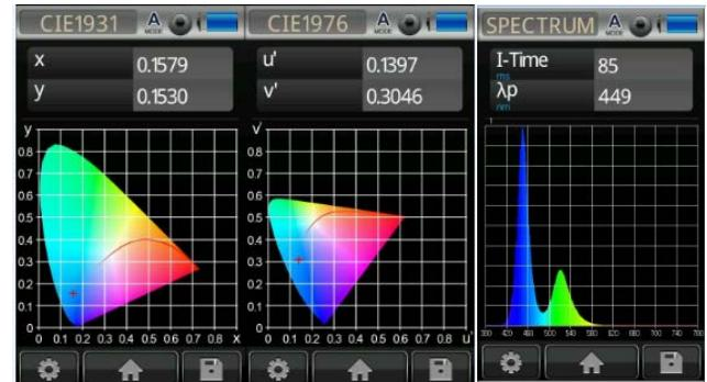
Fig. 3 Spectrum and color coordinates of the projectors used to highlight the vertical outer edges of the building
