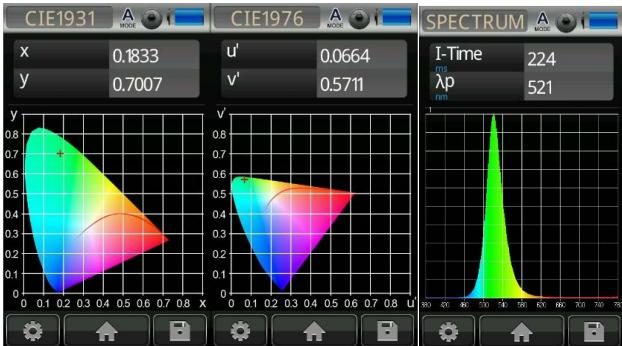
Fig. 5 Spectrum and color coordinates of the flood lights used for the “green” of the Bulgarian flag
