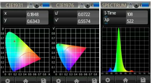
Fig. 7 Spectrum and color coordinates of the flood lights used for the dome and the garden
