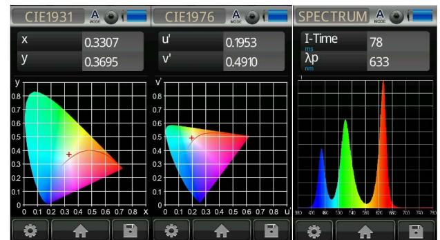
Fig. 4 Spectrum and color coordinates of the flood lights used for the "white" of the Bulgarian flag
