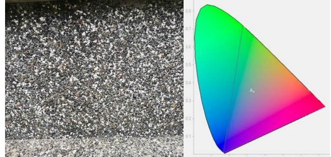
Fig. 7a) Mosaic plaster at the base of the building's façade, b) color coordinates of the plaster in CIE xyY colour space
