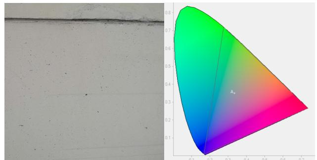
Fig. 3 a) Gipsum based plaster – white, diffuse, b) CIE xyY color coordinates of the plaster
