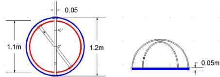
Fig. 3 Gonioreflectancemeter for measurement of BDRF
