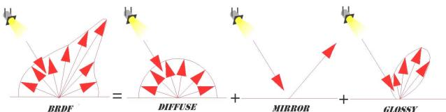
Fig. 2 BRDF of a surface, that has diffuse, mirror and glossy components
