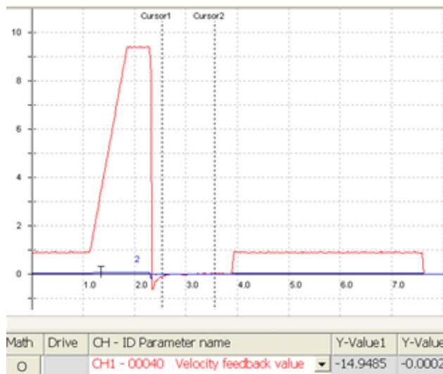
**Figure 5.** Experimentally obtained time diagram for an implemented feed electric drive with AC motor.
