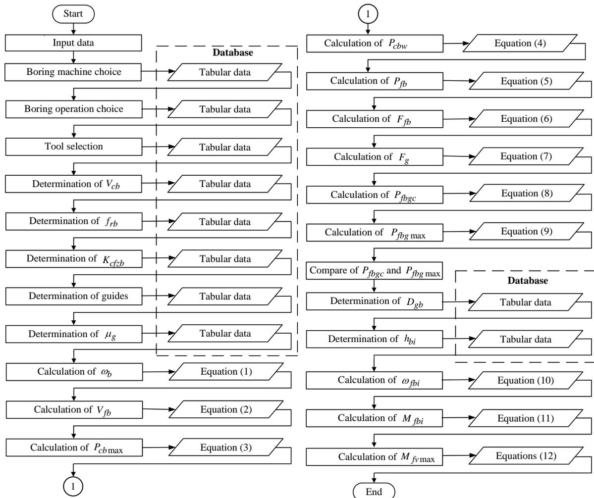
**Figure 2.** Block diagram of the algorithm for drive selection.
