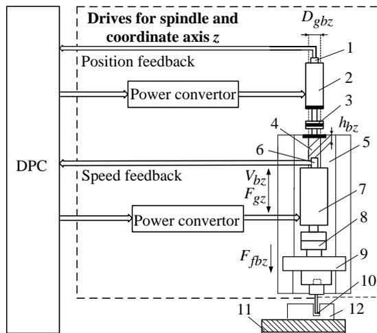
**Figure 3.** Diagram of the elements used for spindle and axis  $z$  drives.
