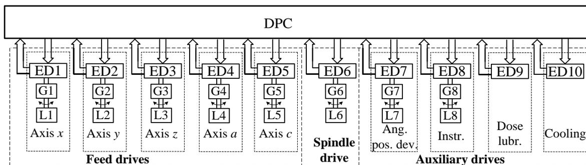
**Figure 1.** Block diagram of the drive system.
