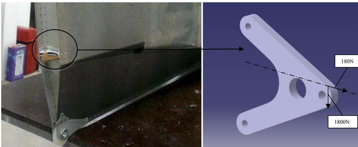
**Figure 1.** A-frame, generated by conventional approach
