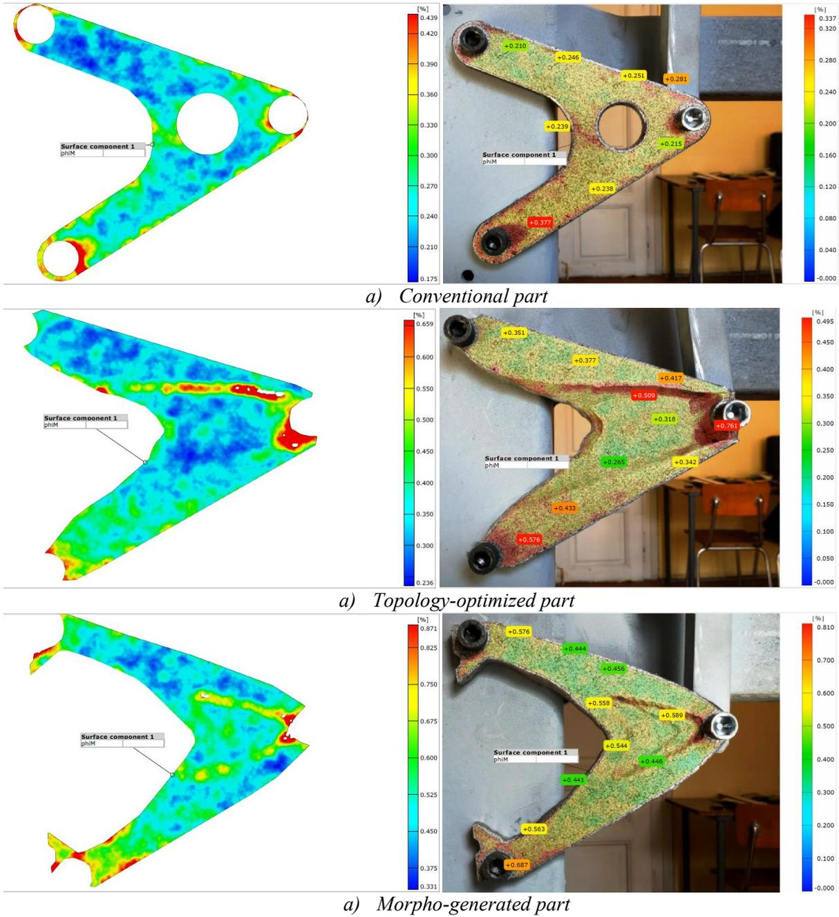
**Figure 6.** Equivalent (von Mises) strains. Without (left) and with (right) original image
