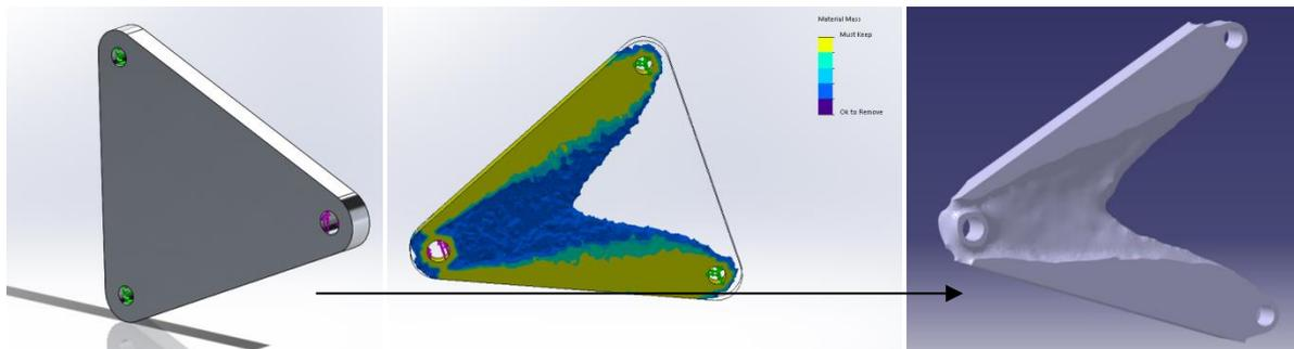
**Figure 2.** Topology-optimized A-frame generated in Solid Works
