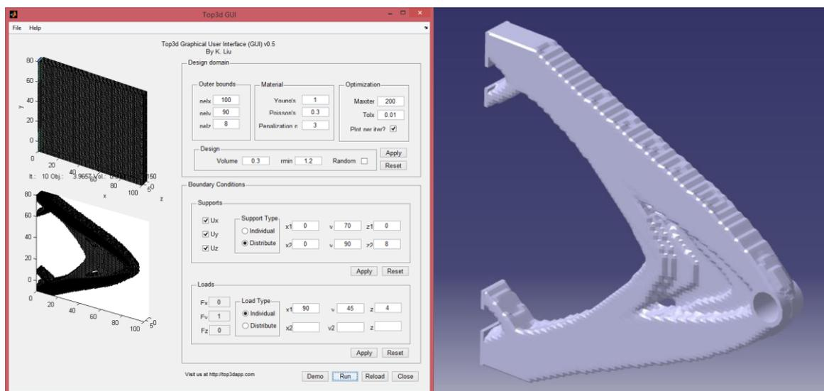
**Figure 3.** Morpho-generated A-frame by Top3D MATLAB optimizer
