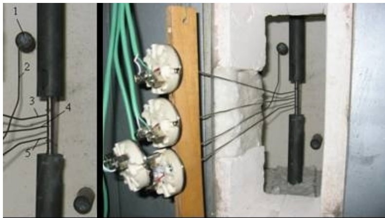
Fig.2 Thermocouples position and numbering
