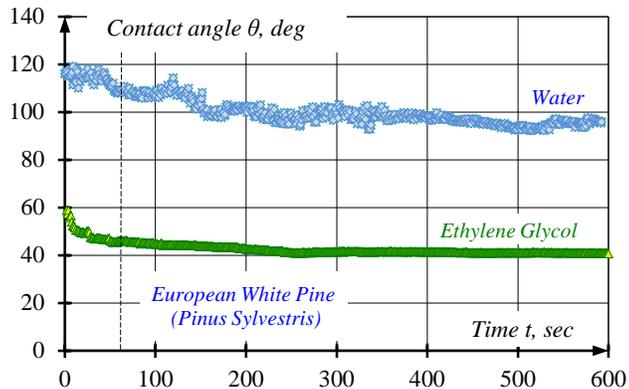
**Fig. 2.** Time-depending change of the contact angle  $\theta$  of probe liquids as well as its slowly advance over the non-ideal European white pine (*Pinus Sylvestris*) bare (non-plasma treated) wood surface.
