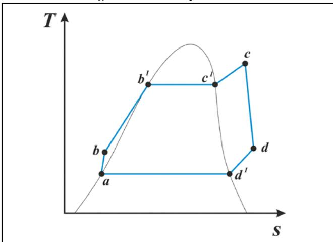
Figure 6. T-S diagram of super-heated RC and ORC
