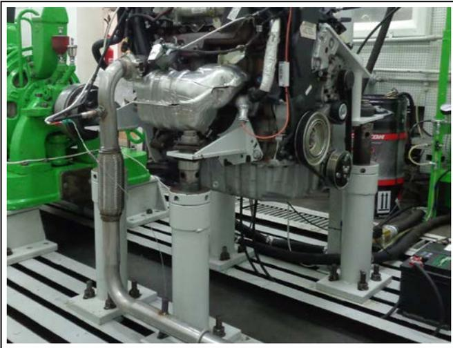
Figure 2. Exhaust temperature sensor position
