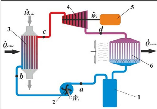
Figure 5. Rankine cycle scheme
