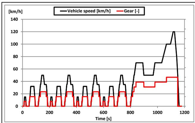
Figure 3. Vehicle speed in NEDC
