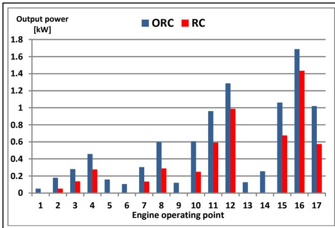
Figure 7. ORC and RC power as a function of engine operating points
