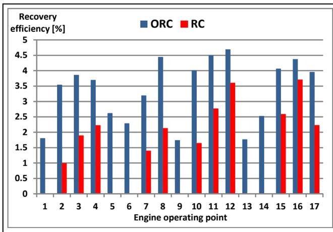
Figure 8. ORC and RC efficiency as a function of engine operating points
