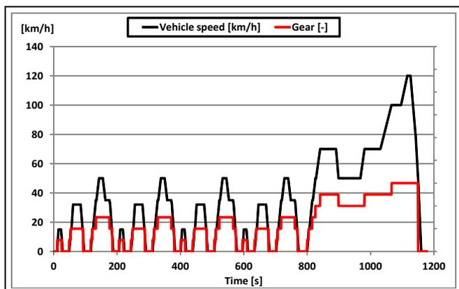
Figure 9. Vehicle speed in NEDC
