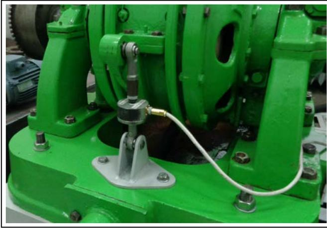
**Figure 2. Brake force sensor**
