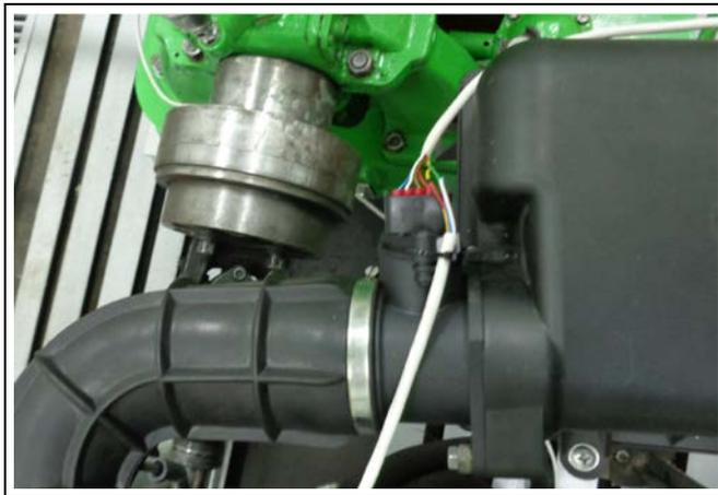
**Figure 3. Intake mass flow meter**
