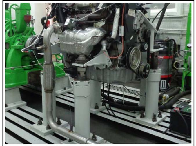
**Figure 5. Exhaust temperature sensor position**
