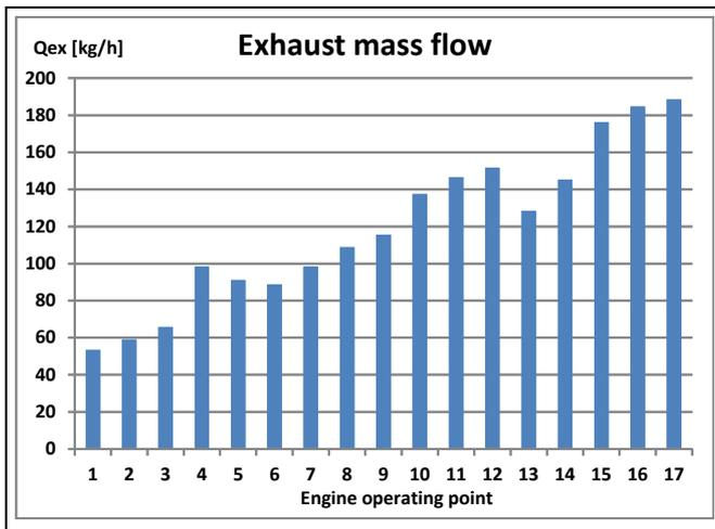
Figure 10. Variation of exhaust mass flow
