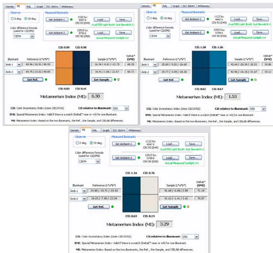
Fig.4 – Results from color stability evaluation of six essential colors from the researched printed design concepts
