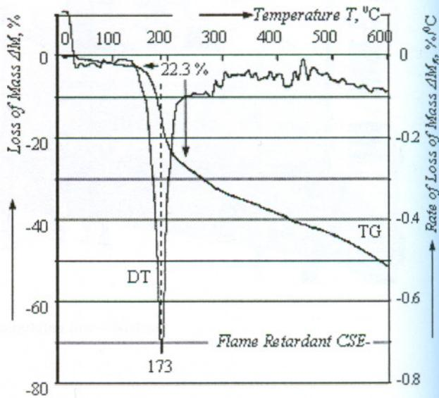
Figure 1. TG and DT thermograms of the flame retardant CSE-96 used (Interiorprotect, Ltd., Bulgaria).
