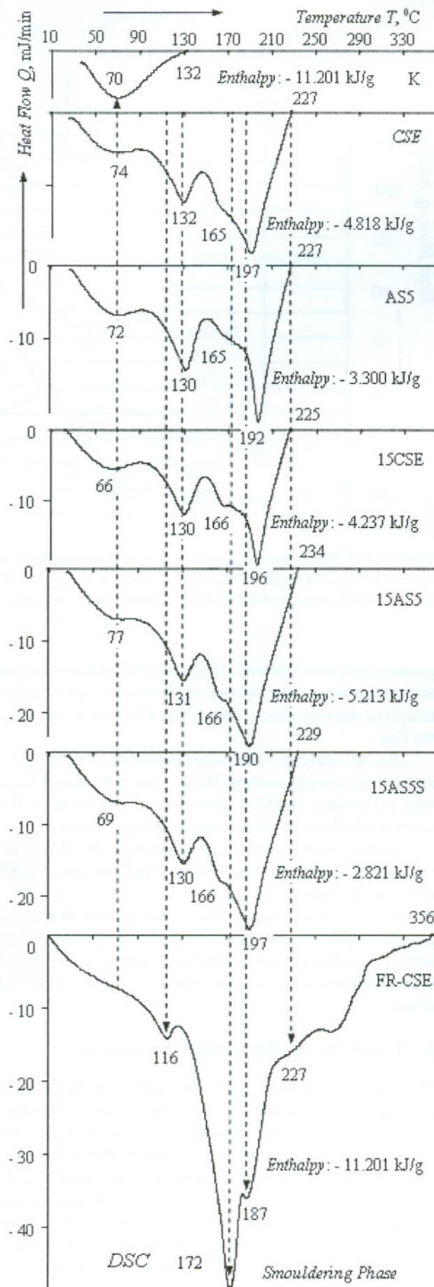
Figure 3. Smouldering and flaming phases of the pyrolysis process; DSC-thermograms illustrating the impact of plasma, surfactant, and spreader on the thermal destruction and combustion of natural and flame retarded wood.
