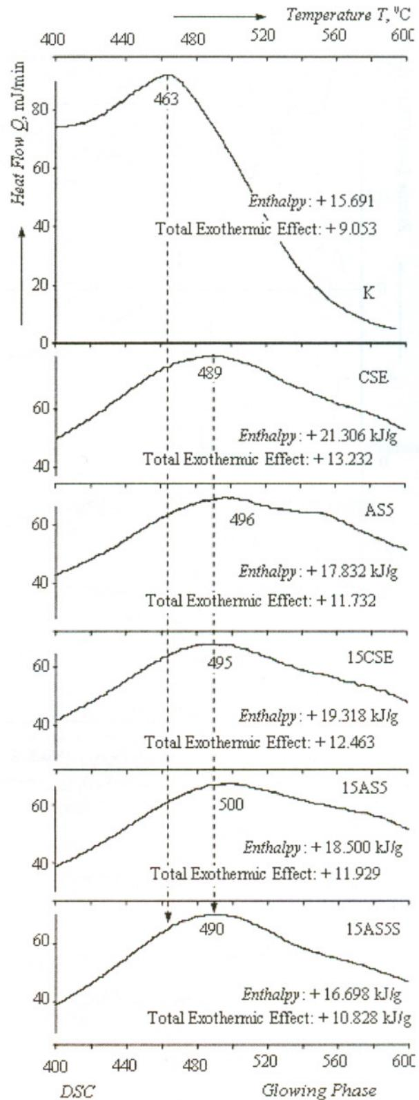
Figure 4. Glowing phase of pyrolysis process - DSC-thermograms; and TG-thermograms of all pyrolysis processes of natural pine wood - K, and different flame retarded woods - CSE, AS5, 15CSE, 15AS5, and 15ASS5.
