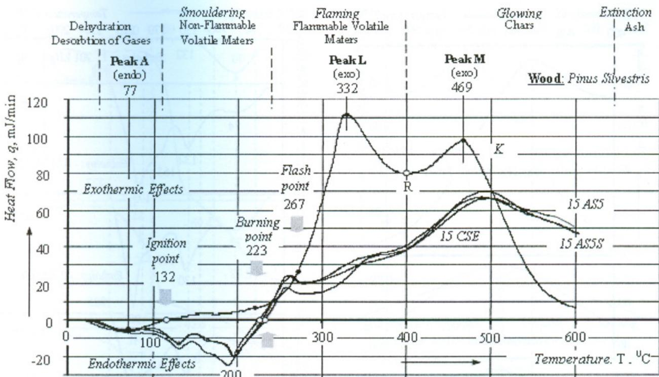
Figure 2. DSC thermograms (heat flow,  $Q$ , versus temperature,  $T$ ) of natural pine (*Pinus sylvestris*) and flame retardant woods, produced by different plasma aided technologies:  $K$  – natural wood; 15CSE – plasma aided capillary impregnation; 15AS5 – plasma and surfactant aided capillary impregnation; 15AS5S – plasma, surfactant, and spreader aided capillary impregnation.
