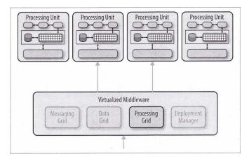
Figure 5. Processing-grid component
