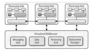
Figure 1. Space-based architecture pattern
