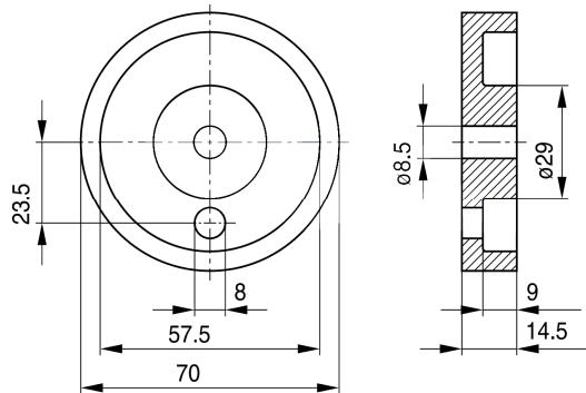
**Figure 2.** The ferrite flux concentrators dimensions.
