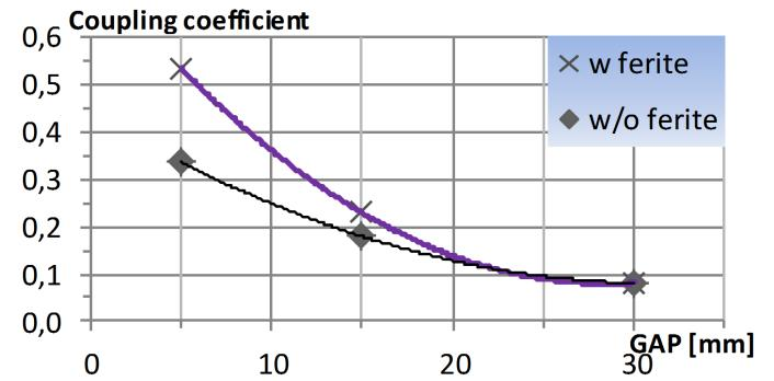
**Figure 7.** Simulated coupling coefficient with (w) and without (w/o) ferrite concentrators
