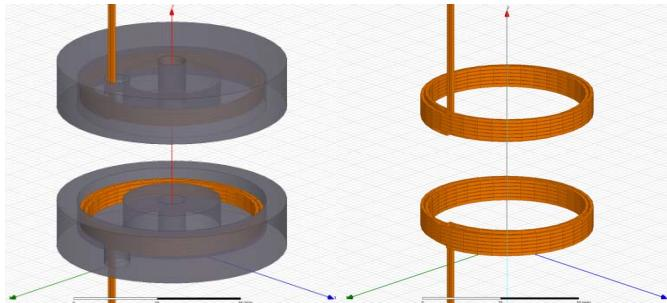
**Figure 1.** The transmitter and receiver design - with and without magnetic flux concentrators.
