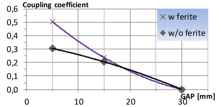
**Figure 8.** Measured coupling coefficient with (w) and without (w/o) ferrite concentrators
