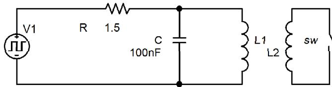
**Figure 6.** Coupling coefficient measurement schematic diagram
