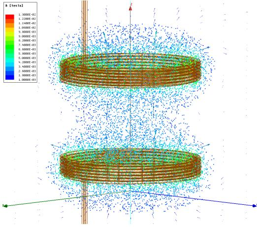
**Figure 9.** Magnetic flux for the coil set without ferrite concentrators
