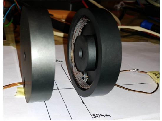
**Figure 4.** Coil set with ferrite magnetic concentrators.
