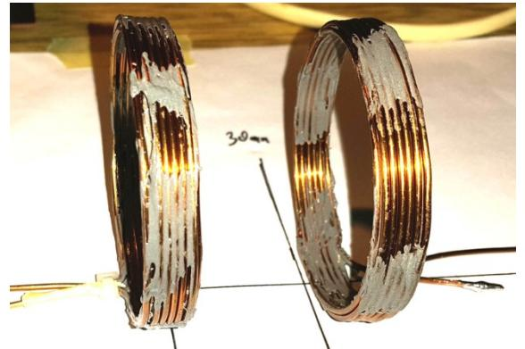
**Figure 3.** Coil set without magnetic concentrators.
