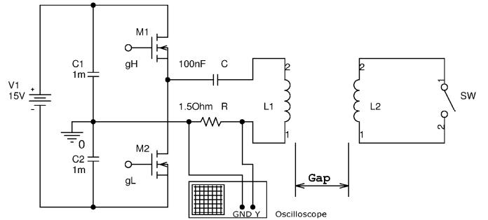
**Figure 5.** Testing setup schematic diagram.
