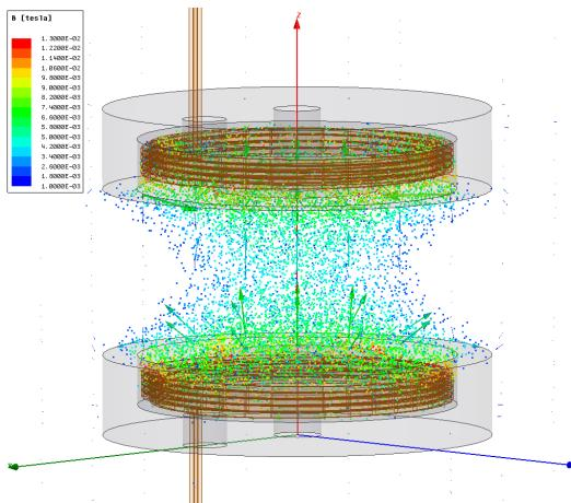
**Figure 10.** Magnetic flux for the coil set with ferrite concentrators
