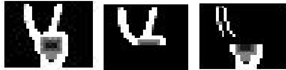
Figure 13. Wrong gesture recognition of a chosen thermal image recognition: on the left - reference gesture; on the middle - variation of the gesture; on the right - image difference between two gestures for which the calculated value of difference is bigger - 0.13, i.e. the recognition is wrong.
