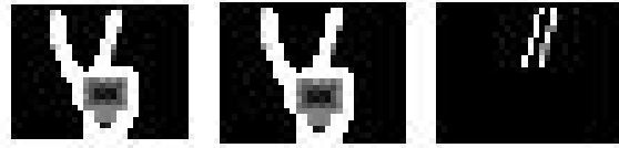
Figure 12. Correct gesture recognition of a chosen thermal image: on the left - reference gesture; on the middle - variation of the same gesture; on the right - image difference between two gestures for which the calculated value of difference is very small - 0.023, i.e. the recognition is correct.
