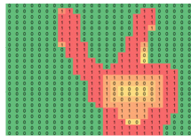
Figure 11. Thermo-visual image (as numerical data shown in pseudo colors) chosen as gesture received from IR – MLX90640 thermo-visual sensor.
