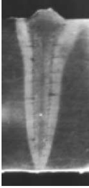
Fig.1. Cross section of the weld ( U_a=60[\text{kV}] ; q=3[\text{kW}] and v=1[\text{cm/s}] )
