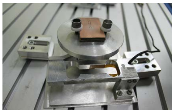
Fig. 2. The device for measurement of torque.
