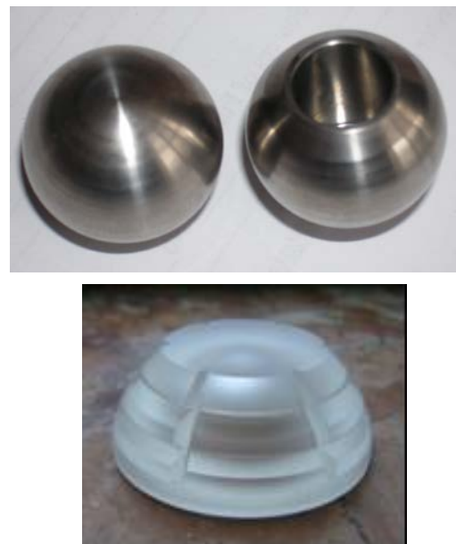
Fig. 3 Experimental specimens of titanium head and sapphire cup for endo-prosthesis of the hip-joint.
