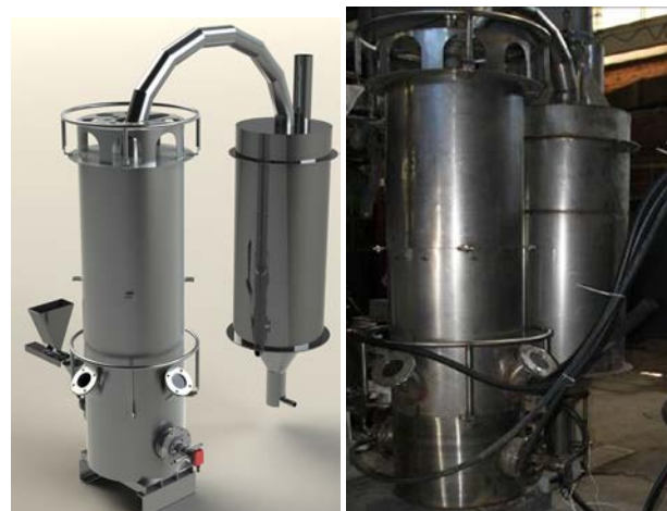
Fig. 1. Pilot unit for TEG generation with a capacity of 8.5 m 3 /h Simulation (left). In metal (right)
