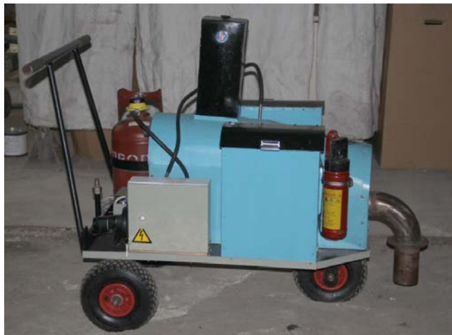
Fig. 2. Autonomous automatic aggregate of a local destination with capacity of 1-2 m 3 /h by TEG
