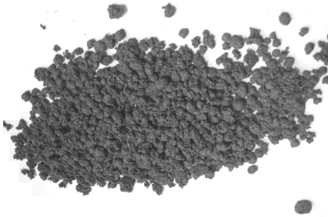
Fig. 5. The granular adsorbent of expanded graphite obtained by extrusion (a) and clumping (b)
