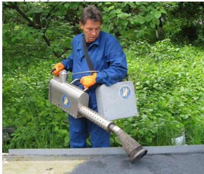
Fig. 3. TEG autonomous knapsack generator with a capacity of 0.8 m 3 /h (3 kg/h by raw material).
