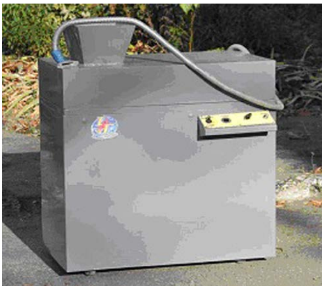
Fig. 7. Experimental unit for the preparation and application of a graphite-aqueous suspension
