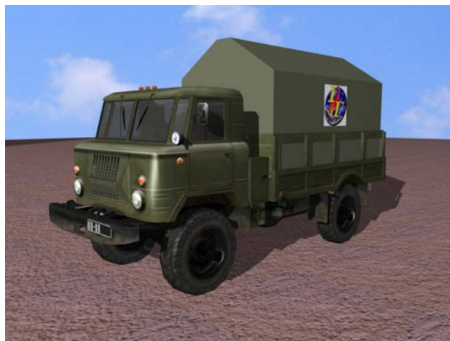
Fig. 4. Mobile unit in a container mounted on a wheeled chassis (truck GAZ-66-02).
