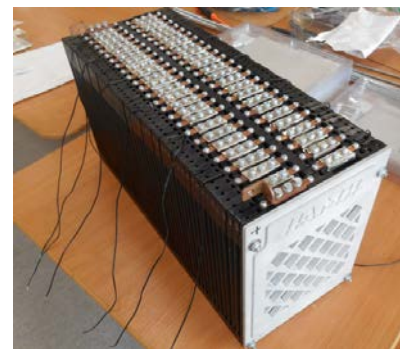
Fig. 7 The experimental sample storage module of the traction battery
