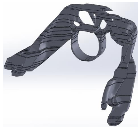
Fig. 8 Partial reconstruction of model B in SolidWorks with loft features
