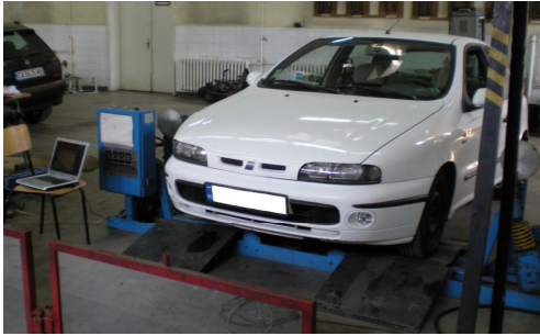
Figure 2. Fiat Bravo on the vibration stand
