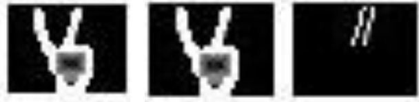
Fig. 8. Correct gesture recognition of a chosen thermal image: on the left - reference gesture; on the middle - variation of the same gesture; on the right - image difference between two gestures for which the calculated value of difference is very small - 0.023, i.e. the recognition is correct.
