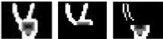
Fig. 9. Wrong gesture recognition of a chosen thermal image recognition: on the left - reference gesture; on the middle - variation of the gesture; on the right - image difference between two gestures for which the calculated value of difference is bigger - 0.13, i.e. the recognition is wrong.
