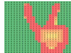
Fig. 7. Thermo-visual image (as numerical data shown in pseudo colors) chosen as gesture received from IR – MLX90640 thermo-visual sensor.
