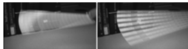
Fig.2 – (left) Smooth blur from flicker free light (right) Stroboscopic effect from flickering lamp
